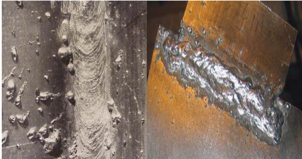
Excessive current - Damp electrodes –Contamination-Incorrect wire feed speed when welding with the MAG welding process-Arc blow
