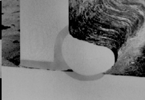
Toe Overlap Fillet weld
